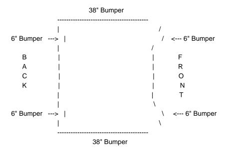
At no point during robot operation does any part of the robot exceed this envelope. On each of the front angled surfaces of the robot we mounted additional 6 inch bumpers as indicated on the diagram. These ensure that the robot makes bumper-to-bumper contact during any collisions as specified in <R08>. All of the bumpers are oriented in a straight-up or vertical position. There is no angle with respect to the vertical.
